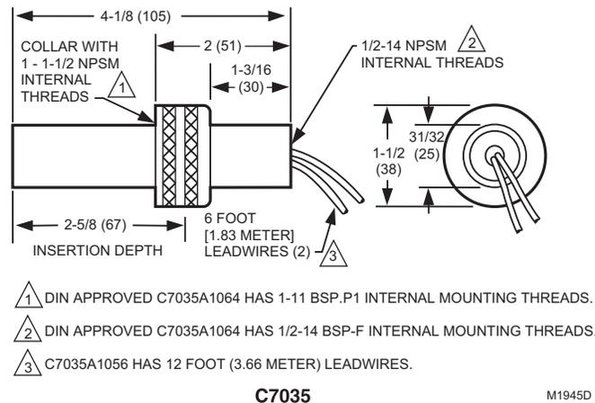
Fig. 2. Installation dimensions of C7035A in in. (mm).
