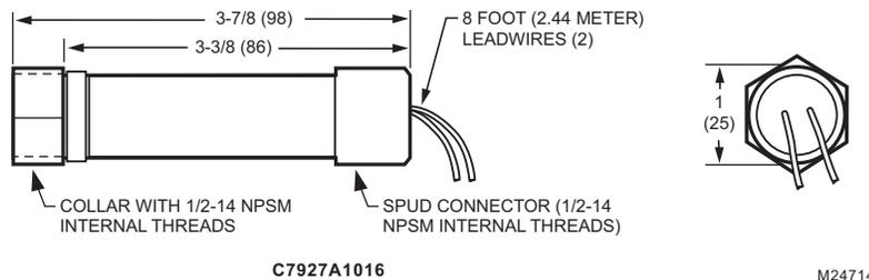
Fig. 4. Installation dimensions of C7927A1016 in in. (mm).
